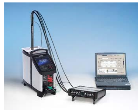
An ASM-803 A connected to the inputs of a JOFRA RTC calibrator, and controlled by JOFRACAL.
