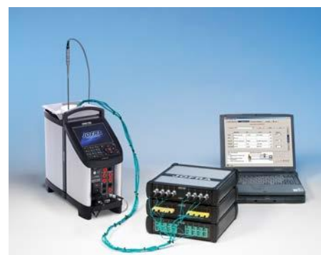
ASM A models connected to the ASM B model, in order to obtain 24 channels. The JOFRA RTC calibrator is used as a dry-block with the reference sensor connected to the reference input of the ATC, all controlled by JOFRACAL.
